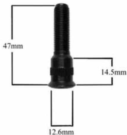
Extended updated (high tensile strength) 3/8 UNF wheel stud 47mm long.
