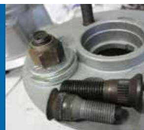
Pulling a wheel stud into place. (Picture extracted from the Triumph Experience Forum.)
